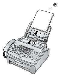
**9** Attach the paper tray cover (①), then push back the tension plate (②).
